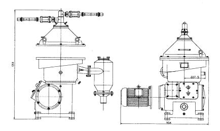
The above projected epitaxial size is the maintenance size for drum, vertical shaft parts and motor-side maintenance spaces, respectively.
